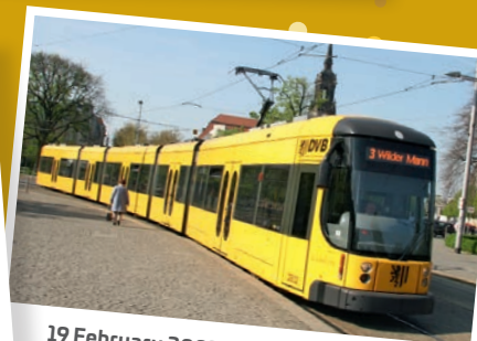
19 February 2003: NGT D12 DD in use At roughly 45 metres, the NGT D12 DD was the longest tram in the world at the time.
