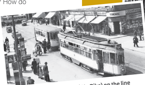
1931: The 'Großer Hecht' (Big Pike) on the line Significant upgrades included the closed driver's cab with a seat for the driver and the two twin-axle bogies.
